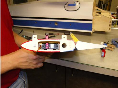
12.As mentioned previously, you may need to adjust the size of the servo arm exit slot to achieve maximum travel. A ¼" Drum sander in a moto-tool makes quick work of this. Repeat these steps for the other stab/elevator half. Before you set aside the stabs take a
