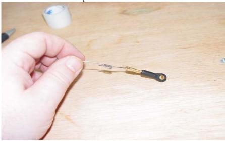
49. Insert the bare end of the cable into the slot in the rear of the fuselage and feed it forward through the hole in the former that is positioned just in from of the slot. Pull the cable forward into the canopy area and make up the same type of linkage as you did previously. Electronically center your servo. Secure the linkage at both ends with a 3mm bolt and nylon insert lock nut. Repeat for the other side. Again, you will want to use a 4 inch arm for the
