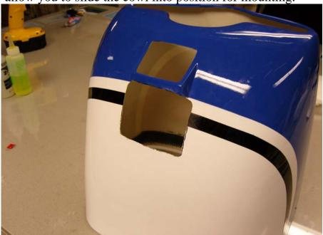
51.Before mounting the cowl place four strips of masking tape on the fuselage as shown and use a felt tipped marker to mark the location of the bolt holes in the cowl mounting tabs. Place the
