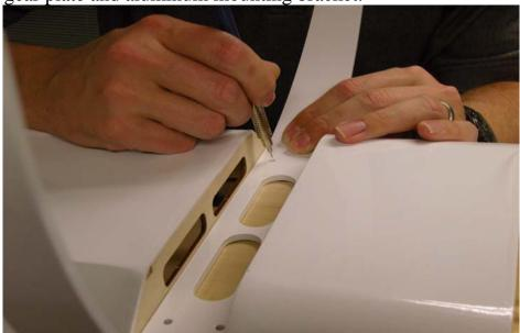
29.Locate the landing gear cover plate and remove the covering from the 2 holes on each end of the cover as shown with a sharp blade.
