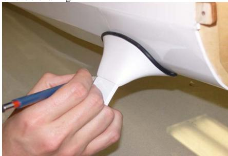
33. Apply a thick bead of silicon glue just above your pencil line all the way around the gear.
