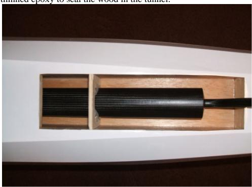
45. A simple plywood mount such as the one pictured works great. Be sure to use silicon tubing to cushion the pipe and prevent it from making contact with the mount.
