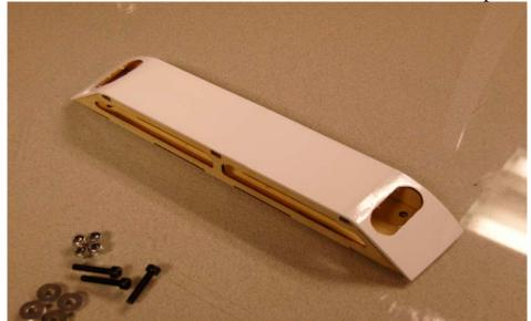
30. Secure the landing gear with 4 4mm bolts, washers and nylon insert lock nuts. Insert the bolts and washers into the landing gear slot cover and into the aluminum landing gear and through the ply
