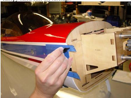
52.Peel the tape back just behind the F1 former and place the cowl into position, flush with the rear of the F1 former. Place your spinner (4") on the engine to aid with alignment. View the cowl from several angles to insure that is positioned properly. When satisfied put the four tape strips back into position and drill a 1/8" hole at the location of each of the 4 ink marks.
