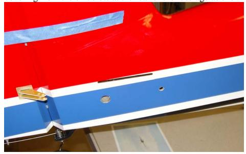
48. Assemble one end of the linkage by inserting the pull-pull cable into a crimp, through the hole in the brass pull-pull fitting and back through the crimp. Loop the cable back through the crimp a second time and crimp with side cutters.
