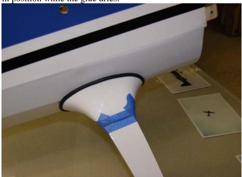
35. Locate the 2 wheel pants and 2 plywood mounting plates. Use sandpaper to scuff the inside of the pant for better glue adhesion. Glue the ply mounting plate centered in the opening of the pant as
