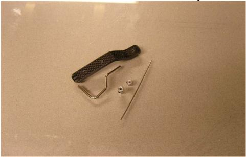
27. Use a rotary tool with a grinding bit or a small file to create a flat spot on the tailwheel wire for the set screws in the aluminum fittings to seat against. Reassemble the unit and apply Loctite to the threads on the setscrews and reinsert into the aluminum fittings and tighten snug. Slide the tailwheel of your choice onto the wire and secure with the 2 included wheel collars.
